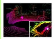
The system can estimate moving vectors of the observation point via sequential 3-D data, and recognize the location in real world in real-time. It can recognize self location for autonomous driving, acquiring the placement of cargo by tracking carriers, and etc.
